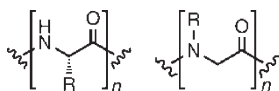
Figure 2. Structures of peptides (left) versus peptoid oligomers (right) (R = side chain). The two structures differ in the location of the R group.
